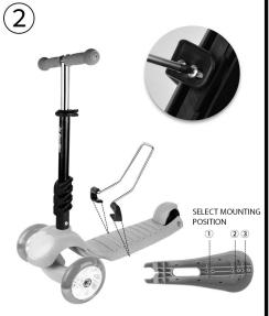
INSTALL THE SEAT BRACKET AND SELECT THE REQUIRED SEAT MOUNTING POSITION
